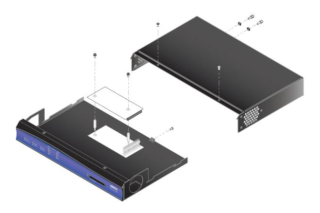
Figure 43. NetVanta Octal PoE Upgrade Installation
